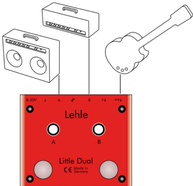
The **Lehle Little Dual** was designed specifically to split and switch the signal of your instrument between 2 amps which are running at the same time. This way you can achieve very nice blends,
