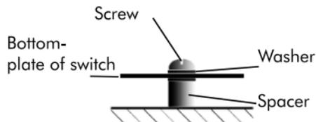
Thanks to its ready-to-go fixing system, the **Lehle Little Dual** can be mounted without difficulty on a base plate. To do this, undo the four housing screws and detach the cover. Then fix the device base to a base plate using the two screws, the washers and the spacers supplied. Replace the cover and tighten the four housing screws - done!
